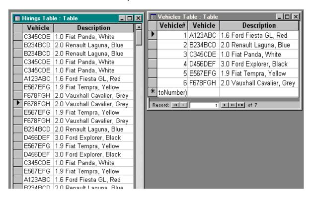
The next step is easy, but tedious. Using *Edit, Replace*, search for each unique occurrence of each record from the *Vehicles Table* as it occurs in the *Hirings Table*, and replace it with the identifying key from the *Vehicles Table*.
